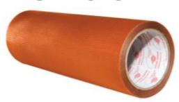
Medium thick film, dark brown creped liner 柔板胶带(褐色皱纹 PVC 离型膜) Double sided mounting tape with PVC backing, for photo polymeric or rubber plates on small diameter cylinders. Immediate high adhesion. No edge lifting even on small cylinders. High flexibility. 双面胶带用于在柔版印刷过程中安装印版。使用专门配制的胶粘剂,不会缠胶。据有高柔然度。
